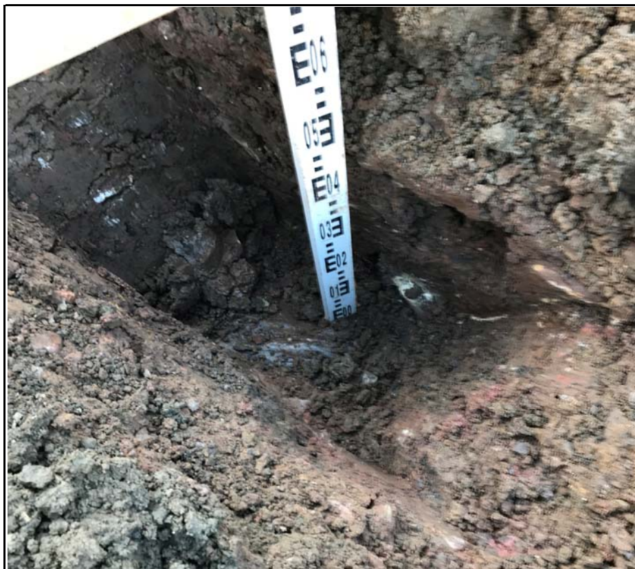
Plot 128 Showing Membrane at Base of Soils
