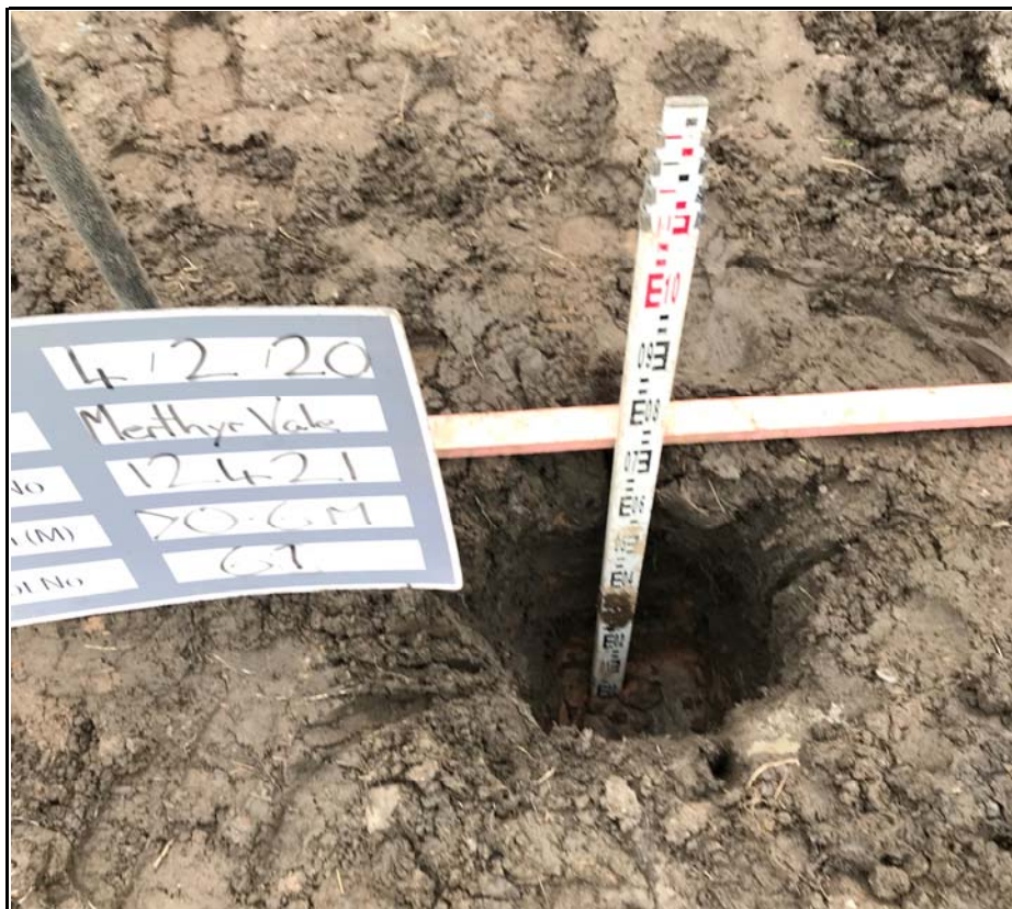
Plot 61 Excavation Pit with Membrane at Base of Soils
