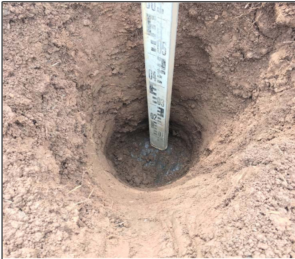
Plot 1 Showing Membrane Placed at Base of Capping
