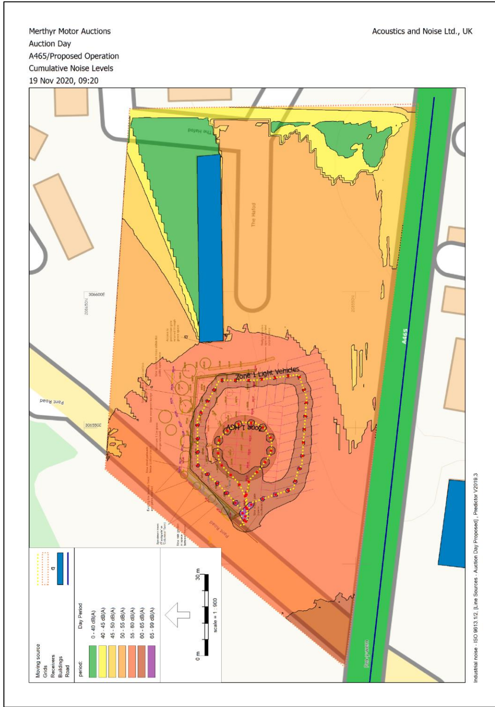
Figure 6 – Cumulative Noise Levels, A465 Road Traffic/Proposed Operations
