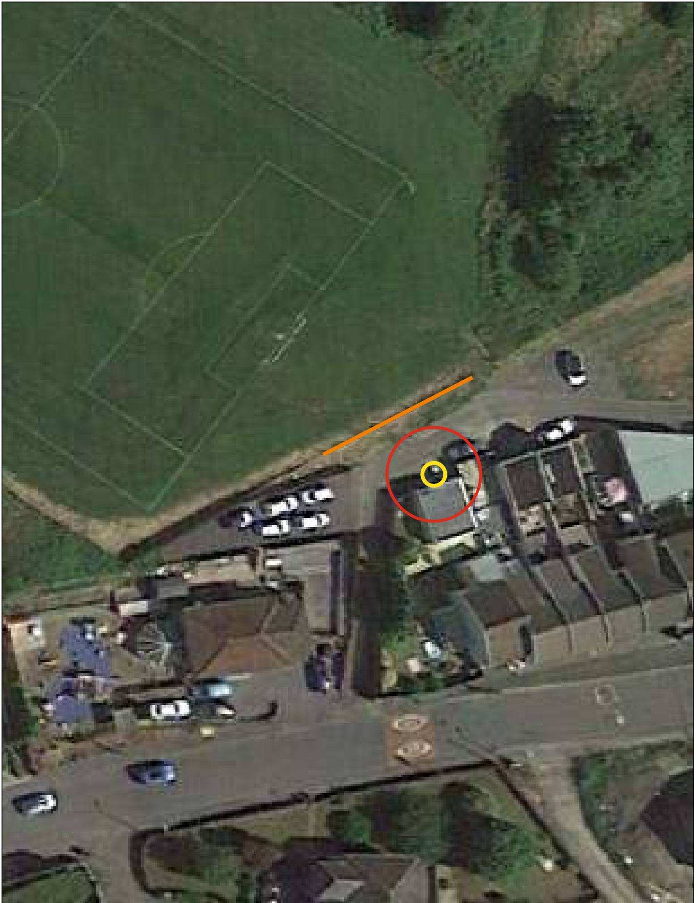
FIGURE 13 SUPPOSED POSITION OF SHAFT 306206-066 ON GOOGLE EARTH IN RELATION TO THE PROPOSED FENCE SHOWN IN ORANGE. A 10m DEPARTURE FOR THE SHAFT POSITION IS SHOWN IN RED.
