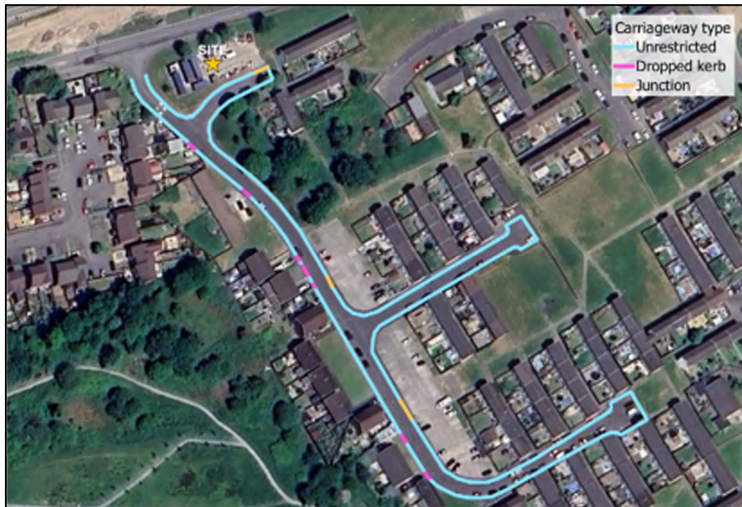
Figure 2.1 On-street parking restrictions
